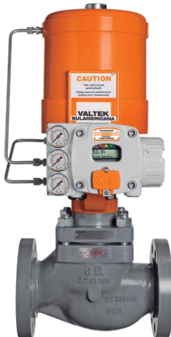
Figure 1: Chronos Positioner Installed in a ValtekSul Globe Valve
